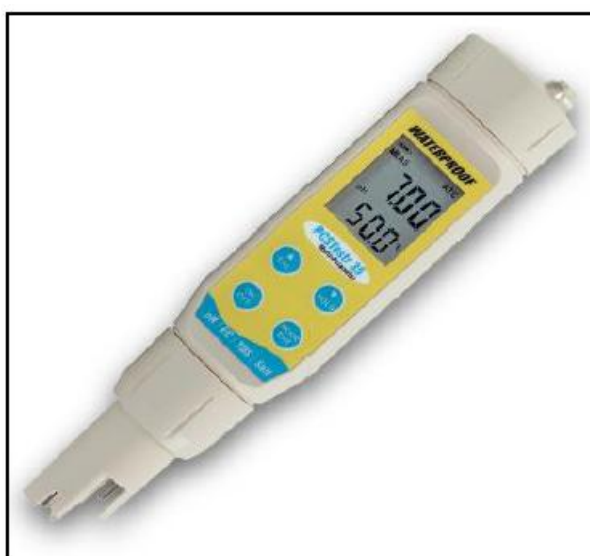
Figure 3.4 Photograph: Multi-Parameter PCSTestr 35
