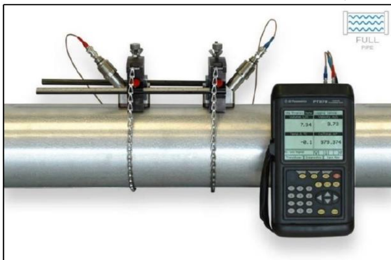
Figure 3.2 Photograph: Clamp on Ultrasonic Water Flowmeter
